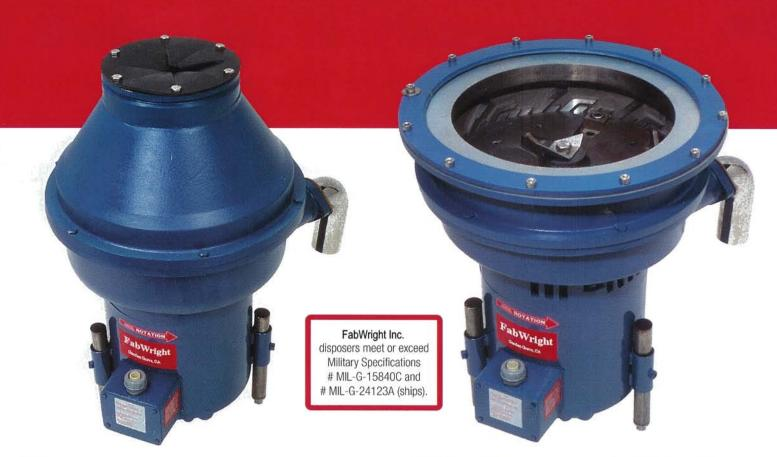
abWright Inc.'s rugged 5 HP, 7.5 HP and 10 HP disposers are designed for operations where waste loads are extreme and volume is heavy. These disposers feature a reduced speed (1140 RPM) to provide optimum performance while finely grinding and disposing of bulky and difficult solid waste such as corn cobs, bones, clam shells, artichoke stems, coconuts, etc. Recommended for operations requiring continuous duty during peak periods for food preparation tables and soiled dish tables.
